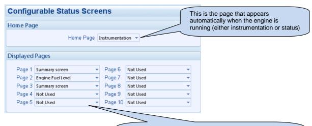
These instruments are displayed one after the other when the set runs. If an entry is set to 'Not Used', or is not applicable, the entry is skipped over and not displayed.
