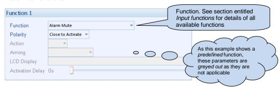
Predefined functions can only be used once in the DSE Configuration Suite. For example if digital input A is configured to 'remote start on load', another input cannot be configured to the same function. Similarly, a PLC function cannot be configured to this function either.
