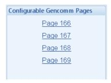
There are 4 configurable Gencomm pages, the user can select which items go into these registers / pages that can be used for PLCs / Building Management systems . This speeds up the communication time as only a limited numbers of registers need to be read instead of poling all the registers within the module that are not necessary used.
