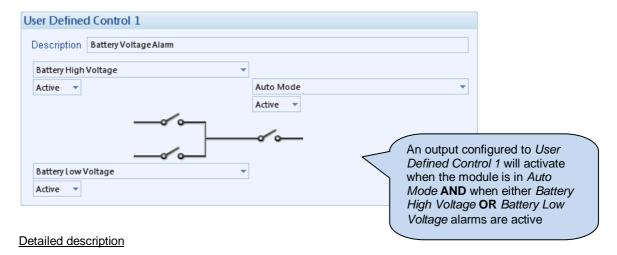
**IF** ( Battery High Voltage alarm is active **OR** the Battery Low Voltage alarm is active ) **AND** the module is in Auto Mode **THEN** the User Defined Control 1 is activated. Any output or LCD indicator configured to User Defined Control 1 will operate.
