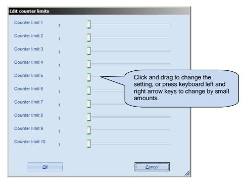
A counter is used by incrementing (adding to) or decrementing (subtracting from) to the counter on the ladder. Upon the counter reaching the configured 'Counter limit', a test for the counter will be successful:
