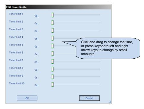
A timer is used by adding the timer action to the ladder. When this action takes place, the timer begins. Upon the timer reaching the configured 'Timer limit', a test for the timer will be successful:
