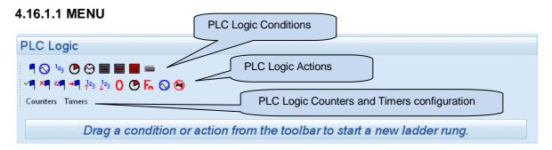
In PLC logic, the ladder of logic is made up of a series of rungs.
