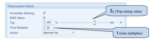
These settings provide for normal use of the mains up to 100% full load. If full load is surpassed, the *Immediate Warning* alarm is triggered, the mains continues to power the load.
