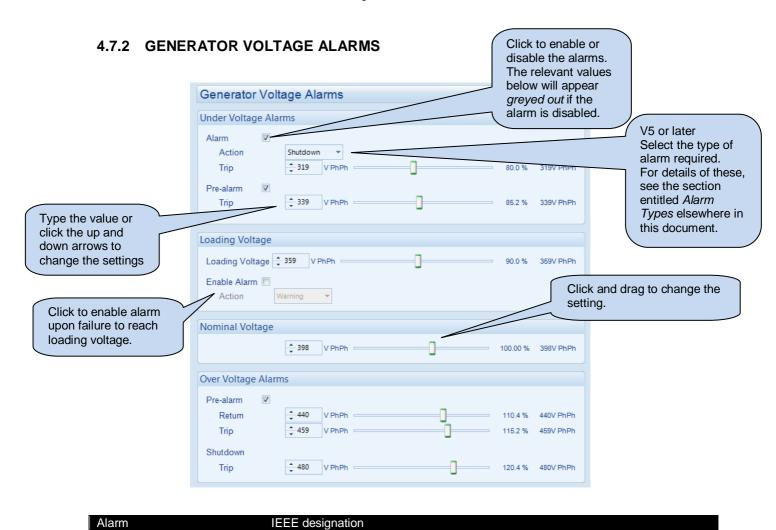
IEEE 37.2 - 27AC Undervoltage relay IEEE 37.2 - 59AC Overvoltage relay
