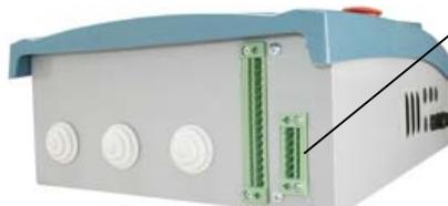
This connector allows customer to remote a general alarm signal or to control the board by remote signals for start and stop by a level sensor. Or, it is possible to block the panel by a switch or EJP or SCR
