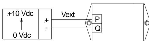
and provide a voltage  $V_{ext} = +5$  V to P and Q terminals.
