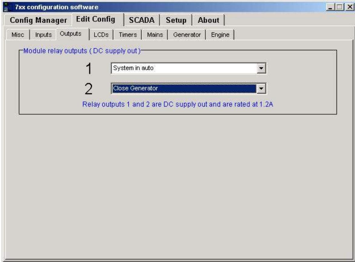
**NOTE:-** The above screenshot shows 720 outputs. Model 710 has 2 additional output relays.
