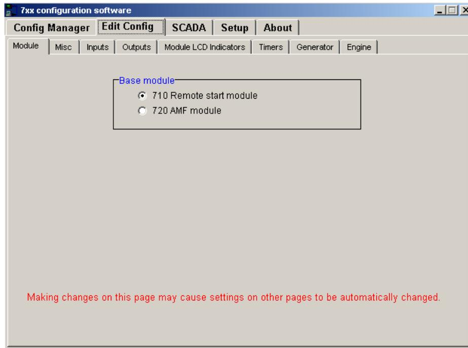
**NOTE:-** It is not possible to write a 710 configuration file to a 720 module and vice versa. However, it is possible to base one configuration on another and select the correct module type on the “module” tab before writing the configuration to the module.
