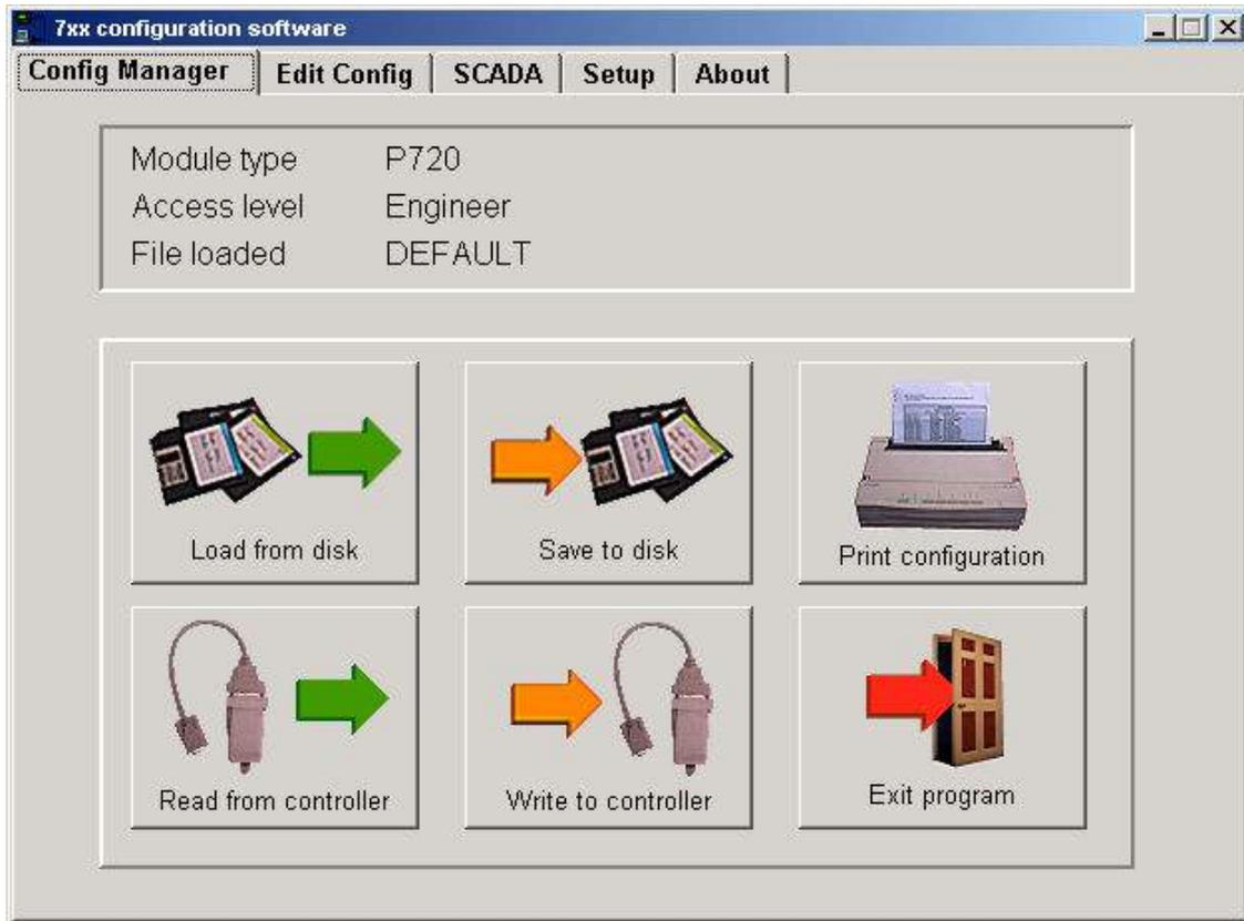
**Module Type:** - This indicates the type of module for which the 7xx series software is currently configured. This will automatically be selected to the correct module when a configuration file is 'Loaded' from disk or 'Read' from the module. It can also be changed under the '*Misc*' tab in the '*Edit Config*' menu.
