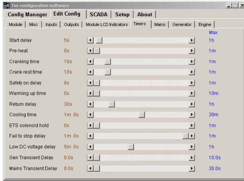
**NOTE:** - Timers can be adjusted by clicking on either the up or down arrow or by clicking on the bar and dragging the bar to the correct time. As the timers can be accurately set to exact times, they can be initially configured with the timers reduced to allow rapid testing of the finished generating set. Once the set is ready for a final witness test, it is just a simple matter of entering the specified timer settings and writing them to the module.
